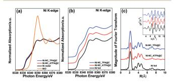
Fig. 2 (a) Ni K-edge X-ray absorption fine structure spectra of Ni-NC\_TPA@C and Ni-NC\_ATPA@C along with those of NiO and Ni foil as reference standards. (b) Enlarged XANES spectra and (c) Fourier transformed EXAFS spectra of the Ni K-edge for Ni-NC\_TPA@C, Ni-NC\_ATPA@C, and Ni foil.
