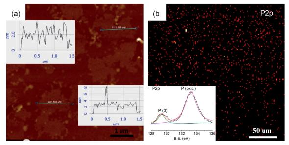
(a) AFM image and height profiles (insets) of thin sheets; (b) XPS mapping and spectrum (inset) of P 2p of thin sheets.
