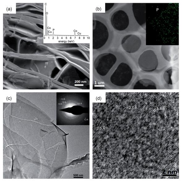
Fig. 5 (a) SEM image and the EDX spectrum (inset) of an irradiated MOFs@P<sub>4</sub> with partial exfoliation; (b) SEM image of a thin sheet and the EDX mapping of the P element (inset); (c) TEM image and SAED spectrum (inset) of thin sheets; (d) HRTEM image of the thin sheet.
