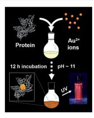
Fig. 1 One-pot protocol for the synthesis of protein (bovine serum albumin)-stabilized luminescent Au clusters.
