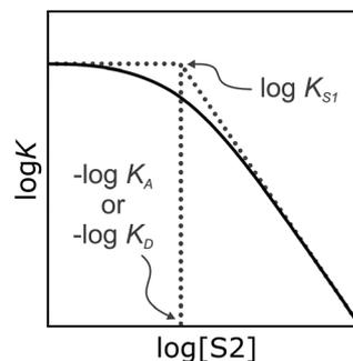
Fig. 2 Dependence of the association constant ( $\log K$ ) for formation of a 1 : 1 complex between a H-bond donor and acceptor on the concentration of a polar solvent (S2) in a non-polar solvent (S1).  $\log K_{S1}$  is the D·A association constant in pure S1, and  $\log K_D$  and  $\log K_A$  are the D·S2 and A·S2 association constants in pure S1.
