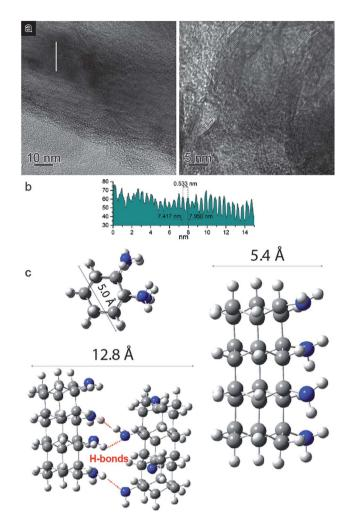
Fig. 4 (a) BF-TEM images at two different magnifications (see inset scale bars) of the recovered material presenting striations spaced at  $\sim$ 4 to 5.1 Å and extending in the longitudinal dimension tens of nanometers. (b) A line profile measured along the white line in the low magnification BF-TEM image (a – left). (c) Views of the optimized DFT geometry structure of the one-dimensional aniline-derived nanothreads with relative dimensions.
