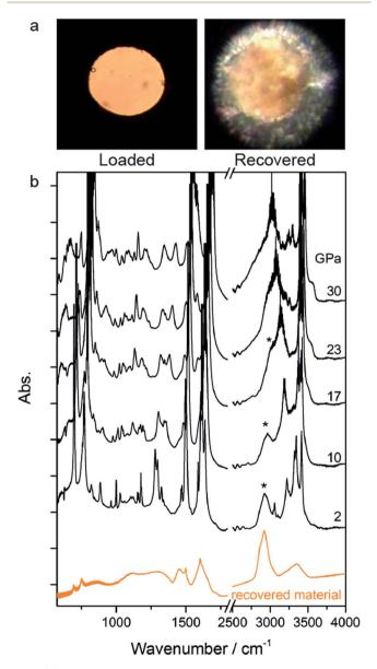
Fig. 3 (a) Optical images of the loaded aniline and the recovered pale yellow/brownish material after decompressing and opening the cell. (b) Infrared absorption spectra for selected pressures recorded along the decompression cycle at 298 K and infrared spectrum of the recovered material, lower trace.
