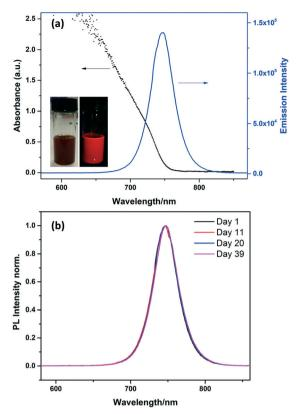
Fig. 3 (a) Absorption and photoluminescence of MAPbI<sub>3</sub> NCs solution in toluene. The insets show the solution under ambient and UV light. (b) PL spectra taken for MAPbl<sub>2</sub> NCs solution over 39 days. The solution was stored in a sealed vial at room temperature in the dark.
