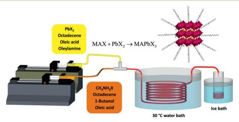
Fig. 1 Schematic diagram of the flow reactor system used for the synthesis of MAPbX<sub>3</sub> nanocrystals at low temperature
