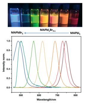
Fig. 4 Photo of sample vials under UV illumination and PL spectra of MAPbl<sub>x</sub>Br<sub>3-x</sub> perovskite NCs in toluene with different halide compositions.
