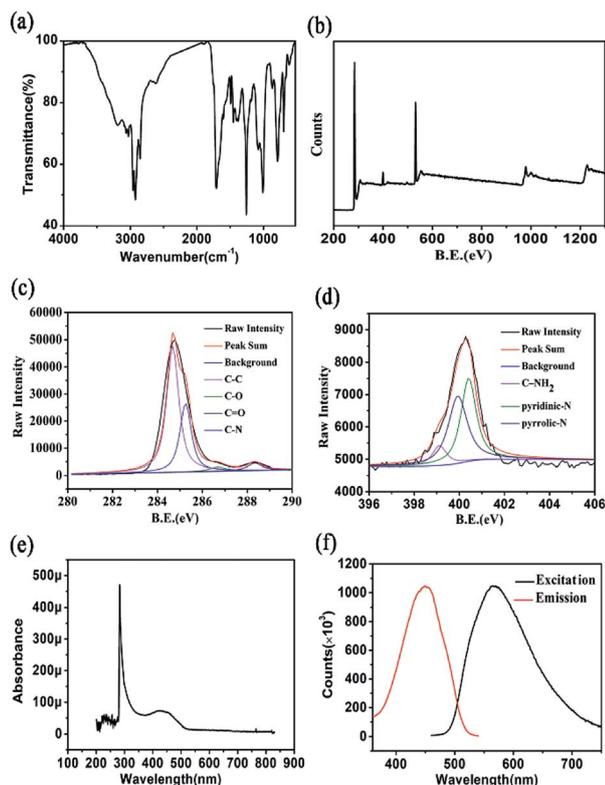
Fig. 3 (a) The FTIR spectrum of the as-prepared CQDs; (b) the survey XPS spectrum of the as-prepared CQDs; (c) high-resolution XPS spectrum of  $C_{1s}$  of the as-prepared CQDs; (d) high-resolution XPS spectrum of  $N_{1s}$  of the as-prepared CQDs; (e) the UV-vis absorption spectrum of the as-prepared CQDs; (f) the fluorescence excitation spectrum and emission spectrum.
