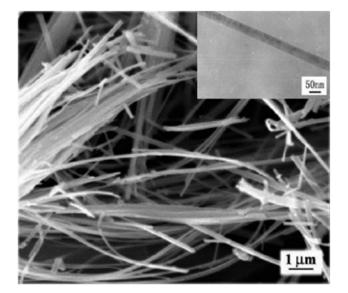
Fig. 8 SEM images of  $TiO_2$  nanowires and a TEM image of a single nanowire prepared by Zhang and colleagues.<sup>135</sup>
