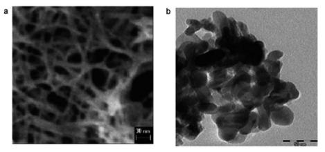
Fig. 9 Electron microscopy images of (a) titania powders and (b) titania nanotubes.<sup>312</sup>
