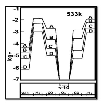
Fig. 4 Influence of gas cycle of sequence on electrical conductivity of 0.5%  $Pt/TiO_2$  doped with (A)  $W^{6+}$  (B)  $Ta^{5+}$  (C) undoped and (D)  $Mg^{2+}$ .85
