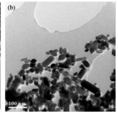
Fig. 7 TEM images of TiO<sub>2</sub> nanoparticles after hydrothermal treatment of TBA peptized gel at (a) 210 °C and (b) 270 °C. 133
