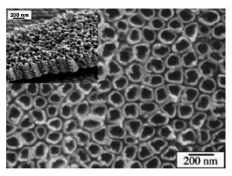
Fig. 13 SEM images of  ${\rm TiO_2}$  nanotubes prepared with anodic oxidation. <sup>159</sup>
