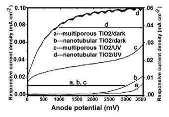
Fig. 18 Measured current of crystallized porous and nanotubular  $TiO_2/Ti$  electrodes under linearly swept potential from 0 to 3500 mV vs. SEC.<sup>217</sup>
