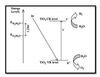
Fig. 17 Mechanism of  $TiO_2$  photocatalytic water-splitting for hydrogen production.  $^{230}$
