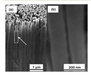
Fig. 6 SEM of  $TiO_2$  nanorods growth in AAM template, (a) low magnification image, (b) high magnification image.<sup>123</sup>
