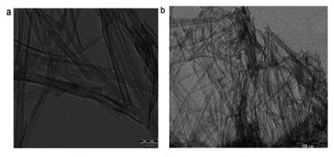
Fig. 10 TEM images of titania nanotubes at (a) low magnification and (b) high magnification. 338
