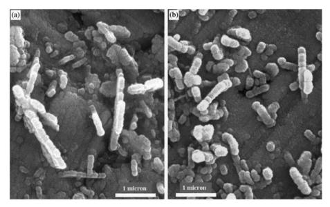
Fig. 14 SEM micrograph of TiO<sub>2</sub> nanowires deposited without NH<sub>3</sub> at 500 °C; (a) with 800 sccm argon flow, and (b) with 500 sccm argon flow. 163
