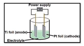
Fig. 11 Depiction of an electrochemical cell in which the Ti samples are anodized. Fabrication variables include temperature, voltage, pH and electrolyte composition.
