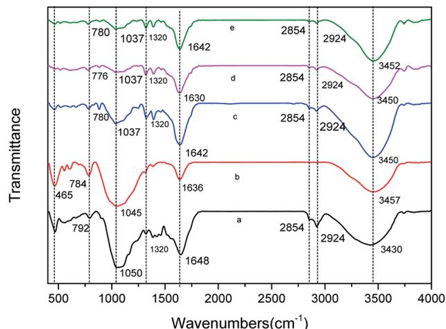
Fig. 1 FTIR of various CMB prepared under different conditions. (a) CMB<sub>200</sub>; (b) CMB<sub>800</sub>; (c) CMB<sub>200-80</sub>; (d) CMB<sub>200-180</sub>; (e) CMB<sub>200-180-w</sub>.
