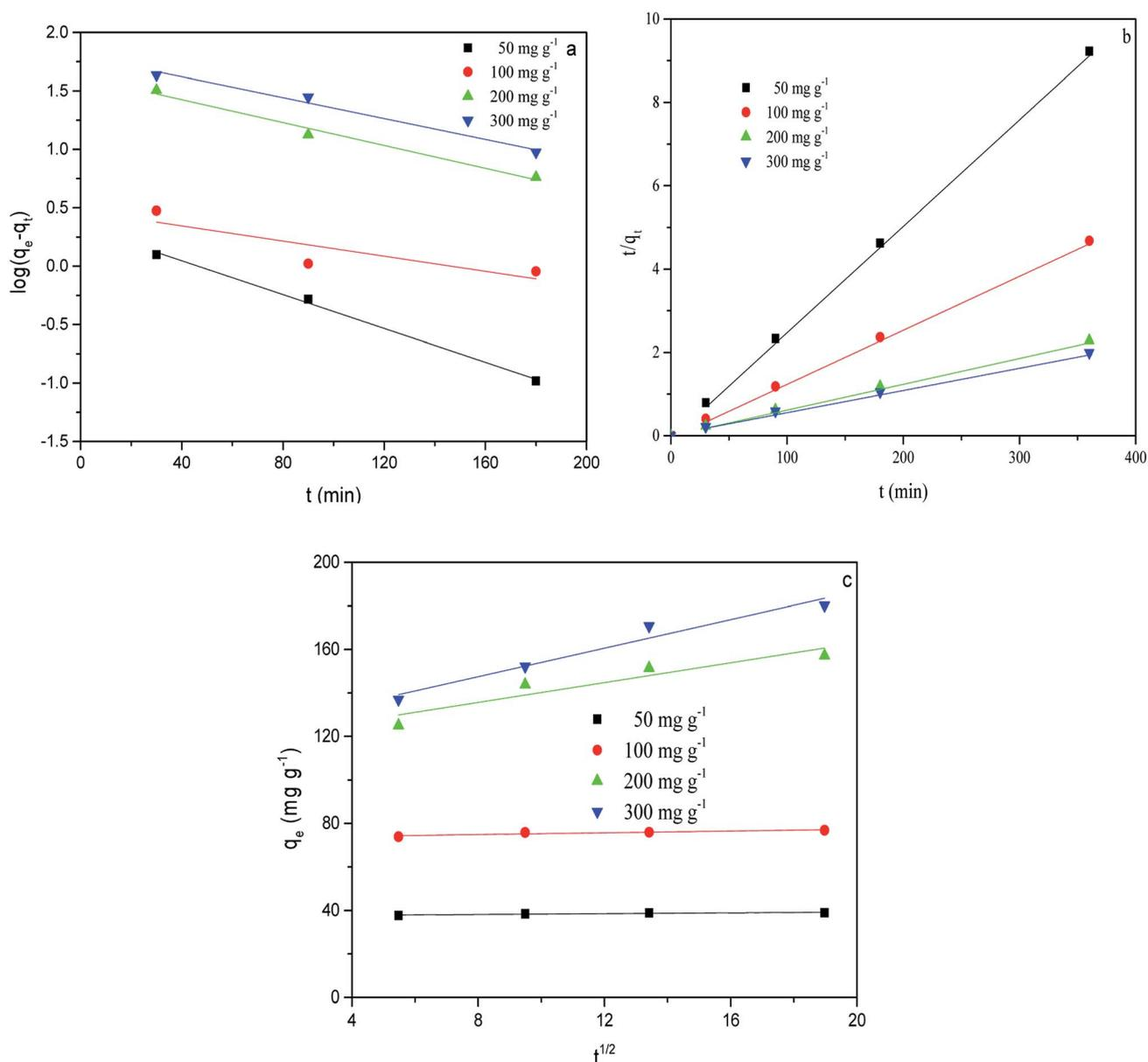
Fig. 9 Kinetic fits for MB adsorption on CMB (25 °C) using different kinetic models. (a) Pseudo-first order; (b) pseudo-second order; (c) intra-particle diffusion.
