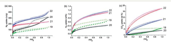
Fig. 10 Gas absorption isotherms of 19-22. (a)  $N_2$  adsorption isotherms at 77 K, (b)  $H_2$  adsorption isotherms at 77 K and (c)  $CO_2$  adsorption isotherms at 273 K and 1 bar. Reproduced from ref. 31 with permission. Copyright© 2015, Royal Society of Chemistry.
