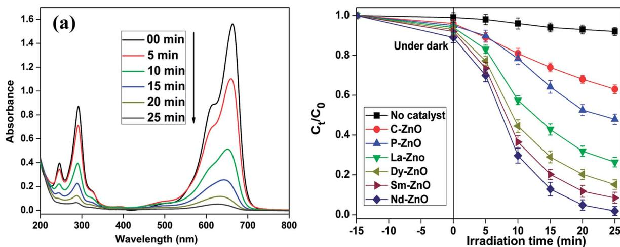
Fig. 8 Decrease in absorption spectra of MB at different time intervals in the presence of Nd-ZnO (a) and change in concentration of MB calculated by following the decrease in  $\lambda_{\text{max}}$  at 663 nm in the presence of different samples under UV-light irradiation (b); catalyst used  $2 \text{ g L}^{-1}$ , pH = 10. Error bars showing the standard deviation of three experiments repeated under analogous conditions.
