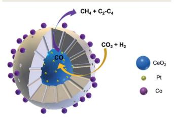
Fig. 10 Schematic diagram of CO<sub>2</sub> hydrogenation on CeO<sub>2</sub>-Pt@mSiO2-Co core-shell catalysts. Reprinted with permission from ref. 118. Copyright 2017 ACS.
