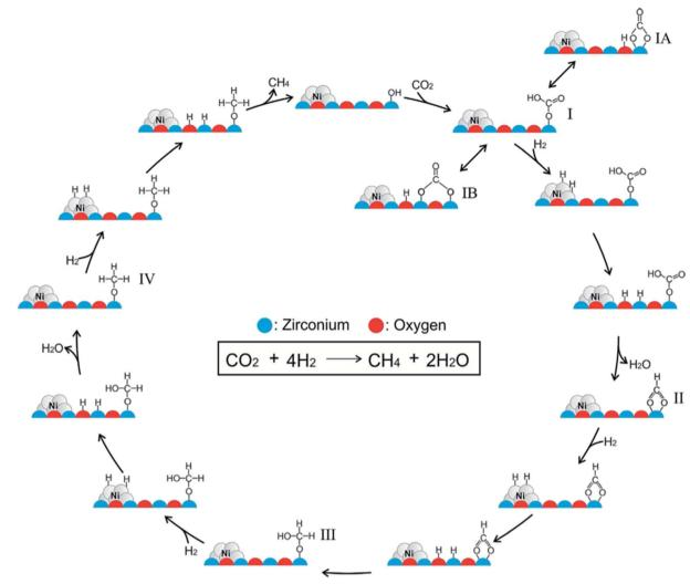
Fig. 8 Mechanism of CO<sub>2</sub> methanation on ZrO<sub>2</sub>-supported Ni catalysts. Reprinted with permission from ref. 99. Copyright 2017 Elsevier.
