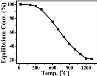
Fig. 3 Equilibrium conversion of  $CO_2$  in methanation at different temperatures (plotted using the data from the literature).<sup>39,40</sup>
