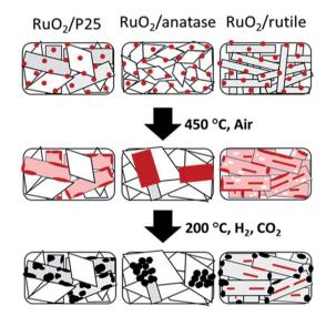
Fig. 5 Schematic illustration of the shape evolution of  $RuO_2/TiO_2$  catalysts: after  $RuO_2$  nanoparticle deposition, after thermal annealing at 450 °C, and after reduction and methanation. Red indicates  $RuO_2$ , pink indicates thin  $RuO_2$  layer, white indicates Ru depleted area, and black indicates metallic Ru. Reprinted with permission from ref. 67. Copyright 2013 RSC.
