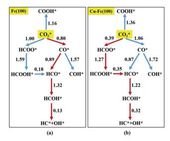
Fig. 12 Reaction networks examined to identify energetically favorable C1 species from  $CO_2$  hydrogenation on (a) Fe(100) and (b) Cu–Fe(100) surface at 4/9 ML Cu coverage. Activation barriers are given in eV (the networks connected with red arrows represent the preferred path for  $CO_2$  conversion to CH\*). Reprinted with permission from ref. 109. Copyright 2017 ACS.
