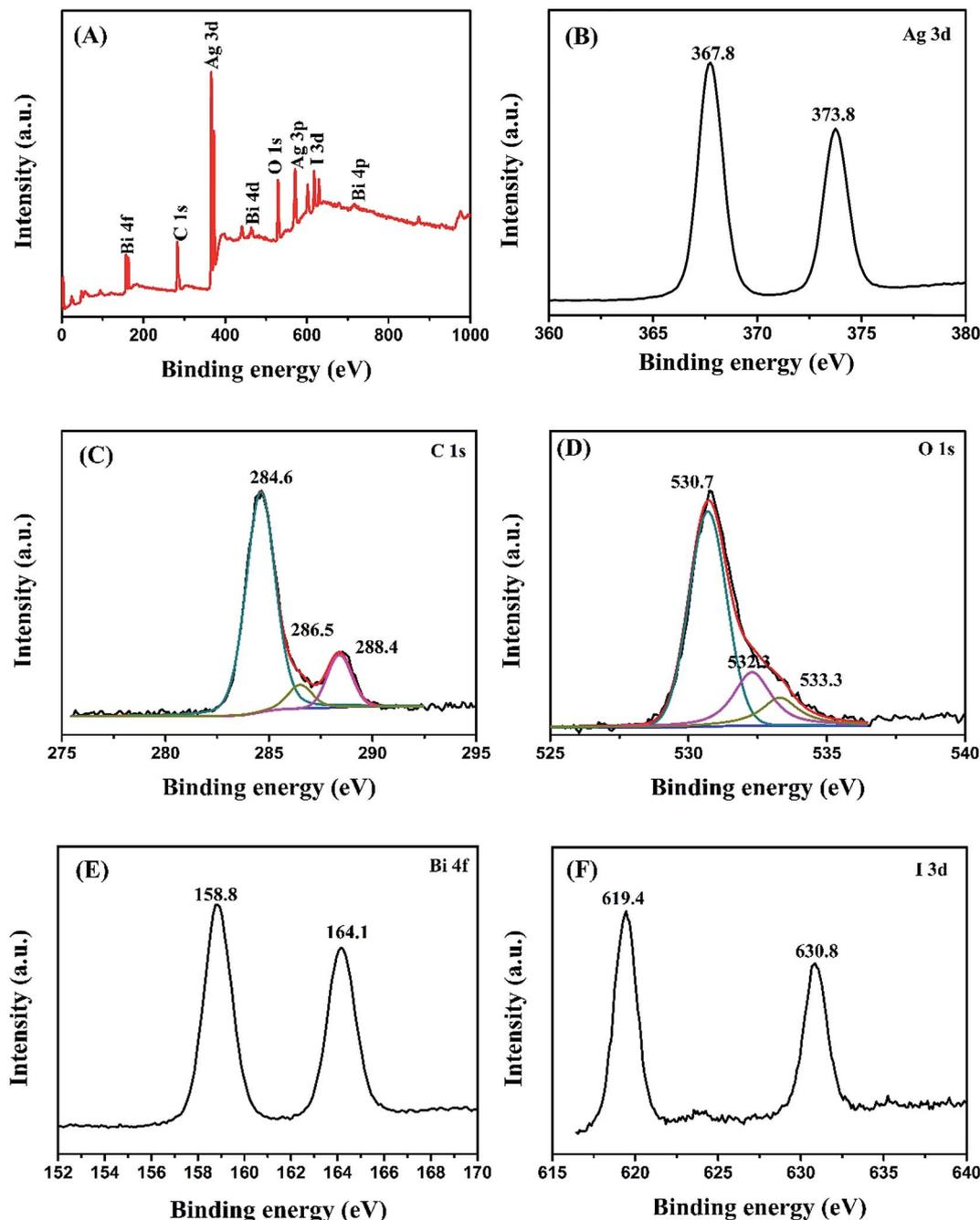
Fig. 3 XPS of BiOI/Ag<sub>2</sub>CO<sub>3</sub> (20 wt%) composite. (A) Survey spectra, (B) Ag 3d, (C) C 1s, (D) O 1s, (E) Bi 4f and (F) I 3d.
