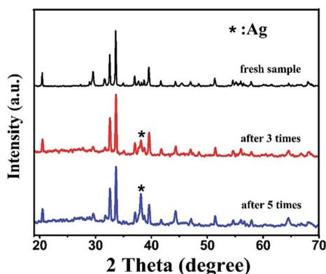
Fig. 10 The XRD patterns of BiOI/Ag<sub>2</sub>CO<sub>3</sub> (20 wt%) composite before and after reuse for photodegrading RhB.
