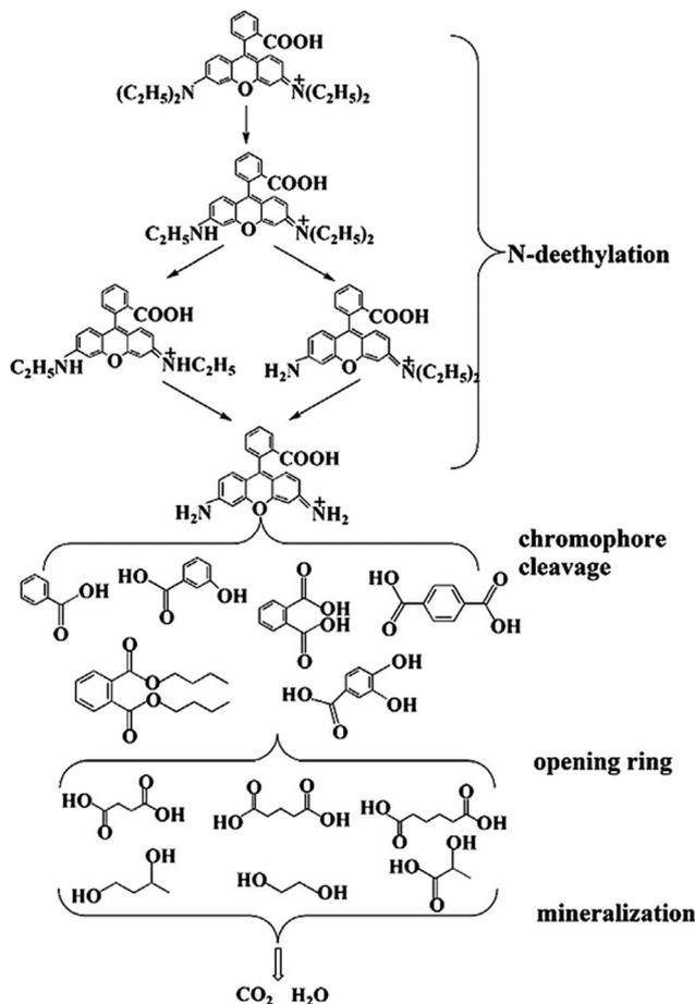
Fig. 13 The possible degradation intermediate and the final products of RhB over BiOI/Ag<sub>2</sub>CO<sub>3</sub> composites.
