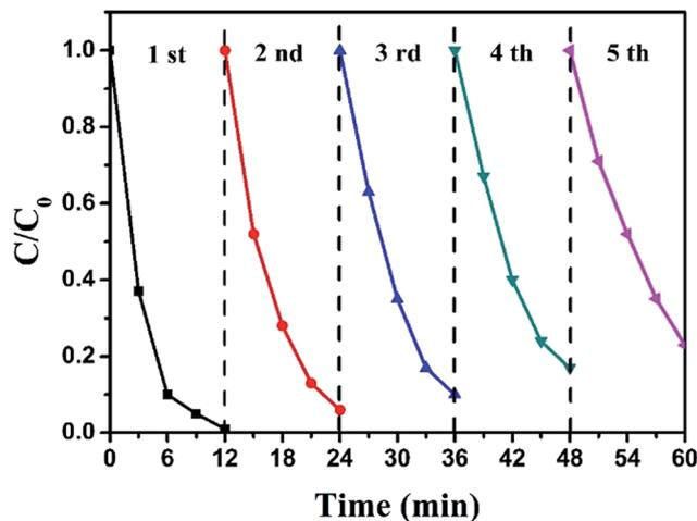
Fig. 9 Recycling experiments for photodegrading RhB over BiOI/Ag<sub>2</sub>CO<sub>3</sub> (20 wt%) composite.
