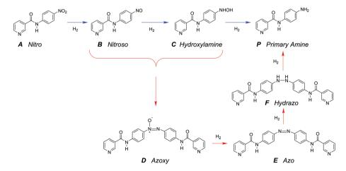
Scheme 2 Proposed reaction scheme. The starting material (A) undergoes reduction to the primary amine by either of two possible reaction pathways: (top) direct hydrogenation to nitroso (B) and hydroxylamine (C) before slow final reduction to primary amine produce (P), or (bottom) condensation of monomeric intermediates to azoxy dimer (D) followed by consecutive reductions and cleavage to the final product amine (P).
