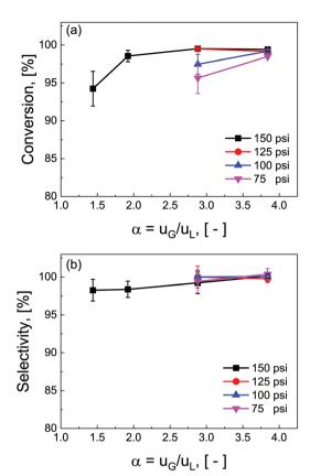
Fig. 3 Multiphase flow optimization. Superficial gas and liquid velocities are screened to achieve maximal (a) conversion, and (b) selectivity at packed bed reactor pressures of 75, 100, 125 and 150 psi. All experiments were conducted at constant liquid flow = 0.4 mL min<sup>-1</sup>. Optimal superficial ratios were at high pressures (150 psi) or large gas flow rates ( $\alpha \ge 1.9$ ).
