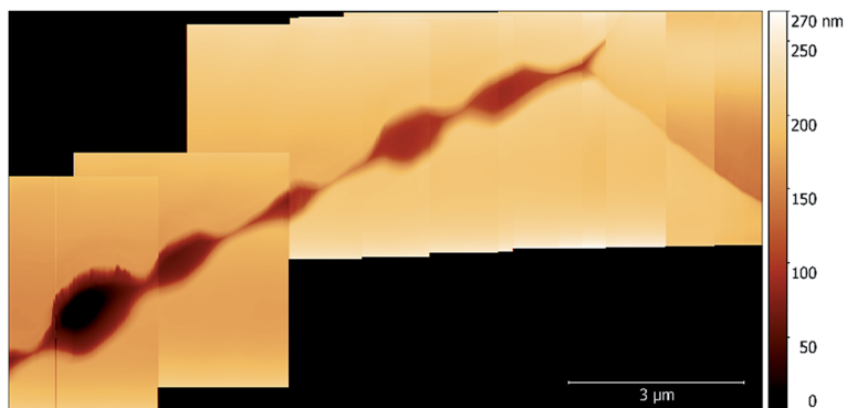
Fig. 6 A topographic map of a number of pits formed along a GB in sensitised AISI 304 stainless steel within 1% aqueous NaCl.
