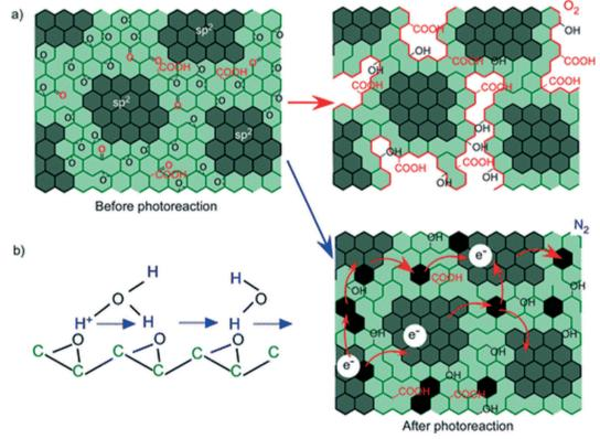
Fig. 23 (a) Models of the pore production by the photoreaction of GO in  $N_2$  and  $O_2$ . (b) Model of proton conduction at epoxide groups.  $^{163}$ Reprinted with permission from ref. 163. Copyright 2012, American Chemical Society.
