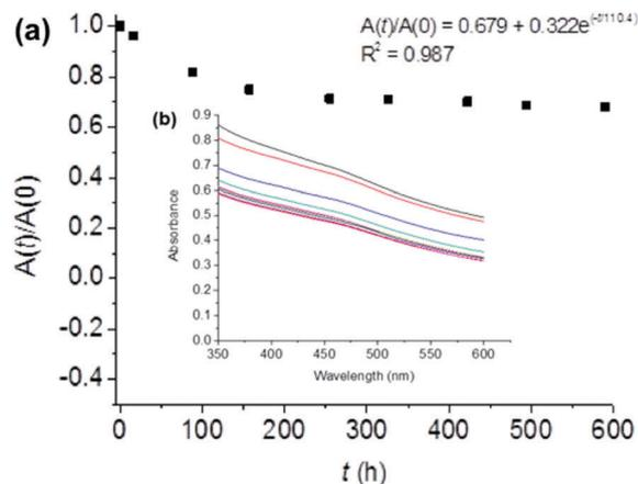
Fig. 3 Stability of BP flakes in solution. (a) The degradation of FL-BP flakes in aqueous 1% w/v Z7950 determined by the ratio of optical absorption at 465 nm at time  $t$  and time zero. The observed lifetime from the fitted decay is around 110 h, whilst ca. 68% of the flakes remains undegraded over a period of ca. 1 month in this media. Inset: Data fitting and  $R^2$ . (b) UV-Vis absorption data used to construct the plot in (a).
