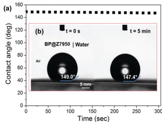
Fig. 4 Contact angle measurements on a PVDF membrane with BP immobilized at the surface. (a) Plot of contact angle ( $^\circ$ ) over time for a drop of deionized water on the BP supported by PVDF membrane. (b) Optical images (CCD camera) of the contact angle of a deionised water droplet on the BP-coated membrane at  $t = 0$  and 5 min.
