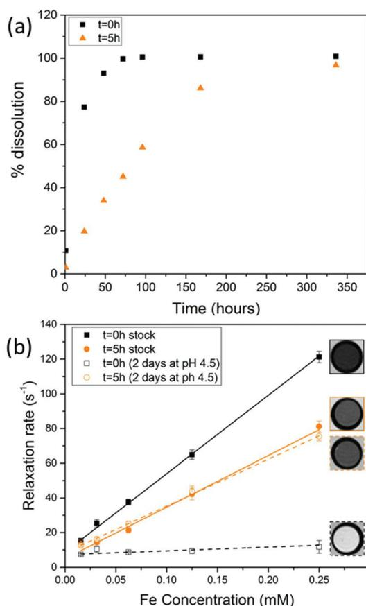
**Fig. 3** (a) Dissolution of SPIONs in citrate buffer system at pH 4.5 at 37 °C for 14 days (b)  $T_2^*$  solution relaxivity of SPIONs before and after exposure to citrate buffer for 2 days. MR images correspond to a concentration of 0.25 mM as imaged with a MGE sequence at TE = 15.5 ms.
