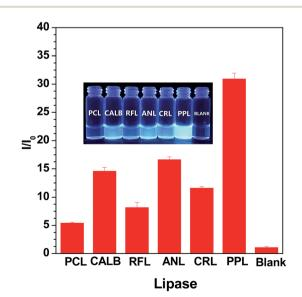
Fig. 3 Plot of the  $I/I_0$  intensity of probe S1 upon the addition of a fixed concentration (80 U L $^{-1}$ ) of commercial lipase samples, respectively, and within an interval of 20 min. The inset shows the corresponding visual fluorescence under UV light illumination at 365 nm. Excitation wavelength: 360 nm.
