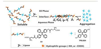
Scheme 1 Schematic illustration of the sensing mechanisms and structure of probe S1 in lipase detection.
