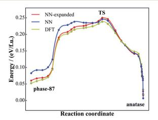
Fig. 7 Minimum energy reaction pathway for the solid-to-solid phase transition from phase-87 to anatase using DFT and NN PES. The reaction coordinate is the relative distance in the generalized coordinate containing both the lattice and atom (see ref. 56 for detail) with respect to the initial state and the final state.
