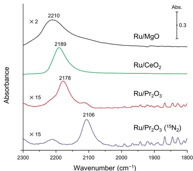
Fig. 6 Difference infrared spectra of N<sub>2</sub> molecules (before and after N<sub>2</sub> adsorption) on supported Ru catalysts. Spectra were collected under 6 kPa of N<sub>2</sub> (<sup>15</sup>N<sub>2</sub> for Ru/Pr<sub>2</sub>O<sub>3</sub>) at 25 °C.
