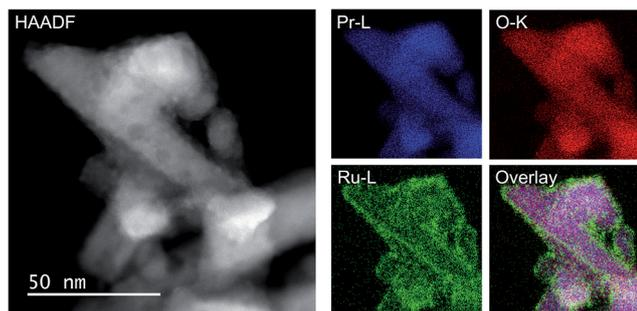
Fig. 3 HAADF-STEM image, Pr-L, O-K, and Ru-L STEM-EDX maps, and reconstructed overlay image of Pr, O, and Ru for Ru/Pr<sub>2</sub>O<sub>3</sub> after H<sub>2</sub> reduction.
