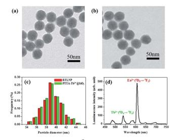
Fig. 3 TEM images of PTTA-Tb<sup>3+</sup>-encapsulated silica particles (a) and RTLNP particles (b). (c) Particle size distribution histograms of the two kinds of nanoparticles. (d) Time-gated emission spectrum of the RTLNP (50  $\mu g$  ml $^{-1}$ ) in 1 : 4 ethanol-0.05 M PBS buffer of pH 7.4 ( $\lambda_{ex}$  = 330 nm).
