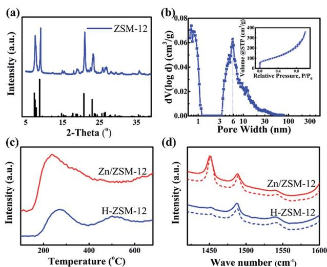
Fig. 2 (a) XRD image and PDF card of H-ZSM-12. (b) BET isothermal curve and pore size distribution of H-ZSM-12. (c) NH<sub>3</sub>-TPD spectrum of H-ZSM-12 and Zn/ZSM-12. (d) Py-IR spectrum of H-ZSM-12 and Zn/ZSM-12. The solid line is the desorption curve at 350 °C and the dashed line is the desorption curve at 200 °C.
