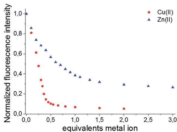
Fig. 4 Fluorescence emission metal titration curve of compound 5 (10  $\mu$ M,  $\lambda_{\text{ex}} = 472$  nm,  $\lambda_{\text{em}} = 552$  nm) using Cu(II) (red  $\bullet$ ) and Zn(II) (blue  $\blacktriangle$ ) in an aqueous sodium cacodylate buffer solution (0.05 M, pH 7.4).
