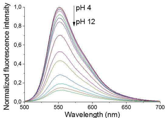
Fig. 1 pH-Dependence of the fluorescent emission spectra of compound 5 (10  $\mu\text{M}$ ,  $\lambda_{\text{ex}} = 472 \text{ nm}$ ) in water.
