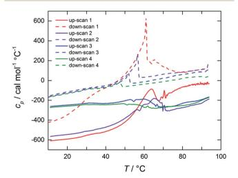
Fig. 6 Raw DSC thermograms of a 10.0 mM NaManLC sample (pH 12.0). Up-scans (solid lines) and down-scans (dashed lines) are obtained with a scan rate of 60  $^{\circ}$ C h<sup>-1</sup> on the same sample.
