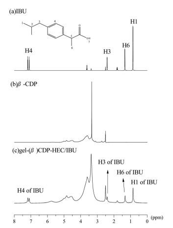
Fig. 10  $\,^{1}$ H NMR spectra of IBU (a),  $\beta$ -CDP (b) and gel-( $\beta$ )CDP-HEC/IBU (c) at 400 MHz in DMSO-d<sub>6</sub> at room temperature.
