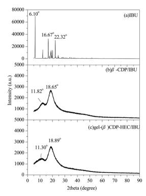
Fig. 12 PXRD spectra of IBU (a),  $\beta\text{-CDP/IBU}$  (b) and gel-( $\beta$ )CDP-HEC/ IBU (c).
