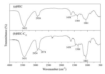
Fig. 2 FTIR spectra of HEC (a) and HEC-C<sub>12</sub> (b).
