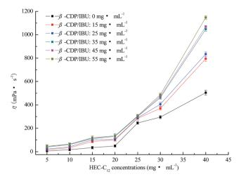
Fig. 8 The dynamic viscosity of gel- $(\beta)$ CDP-HEC at different HEC- $C_{12}$ and β-CDP concentrations.
