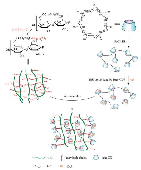
Schematic representation of the formation of self-assembled hydrogels and their drug-loading pattern.
