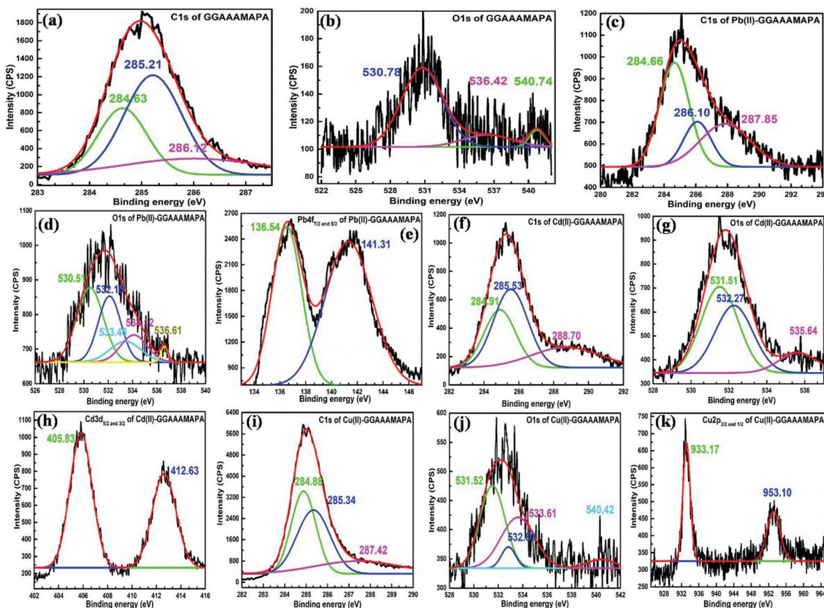
Fig. 5 XPS analyses of C 1s (a, c, f and i), O 1s (b, d, g and j) for GGAAAMAPA and  $\text{Pb}(\text{II})$ ,  $\text{Cd}(\text{II})$  and  $\text{Cu}(\text{II})$  adsorbed GGAAAMAPA;  $\text{Pb} 4f_{7/2}$  and  $5/2$  (e),  $\text{Cd} 3d_{5/2}$  and  $3/2$  (h) and  $\text{Cu} 2p_{3/2}$  and  $1/2$  (k) of  $\text{Pb}(\text{II})$ ,  $\text{Cd}(\text{II})$  and  $\text{Cu}(\text{II})$  adsorbed GGAAAMAPA, respectively.
