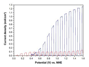
Fig. 10 Chopped light current–potential curves of cold sprayed  $WO_3$  (blue) and  $TiO_2$  (red) on titanium metal photoanodes in 0.5 M  $H_2SO_4$  with a scan rate of 20 mV s<sup>-1</sup>. Current densities were measured upon irradiation with AM 1.5-global light (300 W Xe lamp).
