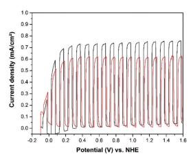
Fig. 7 Chopped light current–potential curves of cold sprayed  $\text{TiO}_2$  on titanium metal (red) and screen printed  $\text{TiO}_2$  on FTO (black) photo-anodes in 0.5 M  $\text{H}_2\text{SO}_4$  with addition of 10 vol% of methanol (~2 mol L<sup>-1</sup>). Measured with a scan rate of 20 mV s<sup>-1</sup>. Current densities were measured upon irradiation with AM 1.5-global light (300 W Xe lamp).
