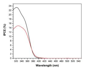
Fig. 8 IPCE spectra for water oxidation measured for cold sprayed  $TiO_2$  on titanium metal (red) and screen printed  $TiO_2$  on FTO (black) photo-anodes. Measurements for water oxidation were conducted in an aqueous 0.5 M  $H_2SO_4$  solution at a bias of 1 V vs. NHE.
