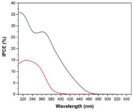
Fig. 13 IPCE spectra for water oxidation employing cold sprayed  $WO_3$  (blue) and  $TiO_2$  (red) on titanium metal photoanodes. Measurements for water oxidation were conducted in an aqueous 0.5 M  $H_2SO_4$  solution at a bias of 1 V vs. NHE.
