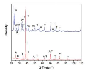
Fig. 2 XRD patterns of  $WO_3$  (blue) and  $TiO_2$  (red) films deposited on titanium metal substrates by cold spray, where W denotes the  $WO_3$  pattern, T the titanium metal pattern, R the rutile  $TiO_2$  pattern and A the anatase  $TiO_2$  pattern.
