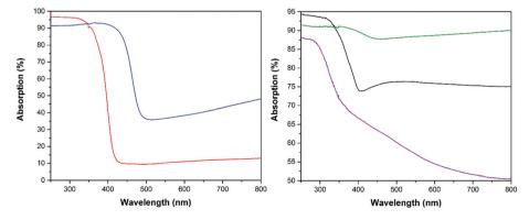
Fig. 3 Absorption spectra of the employed  $WO_3$  (blue) and  $TiO_2$  P25/20 (red) powders (left side) and of the cold sprayed  $Ti/WO_3$  (green) and  $Ti/TiO_2$  (black) photoelectrodes (right side). The purple curve on the right side shows the absorption spectra of the employed blank Ti substrate.
