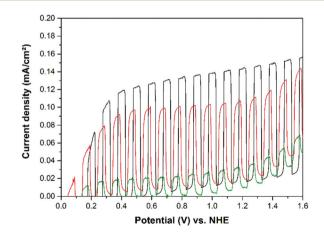
Fig. 6 Chopped light current-potential curves of cold sprayed TiO<sub>2</sub> on titanium metal (red), screen printed TiO2 on FTO (black) and screen printed TiO<sub>2</sub> on titanium metal (green) photoanodes in 0.5 M H<sub>2</sub>SO<sub>4</sub> recorded with a scan rate of 20 mV s<sup>-1</sup>. Current densities were measured upon irradiation with AM 1.5-global light (300 W Xe lamp).
