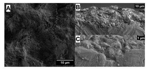
Fig. 4 (A) SEM surface morphology image of a cold sprayed TiO<sub>2</sub> film. (B) Cross-sectional SEM image of a cold sprayed WO<sub>3</sub> film on a titanium substrate at a magnification of 1400x. (C) Cross-sectional SEM image of the interface between the cold sprayed WO<sub>3</sub> film and the titanium substrate at a magnification of 8500x.
