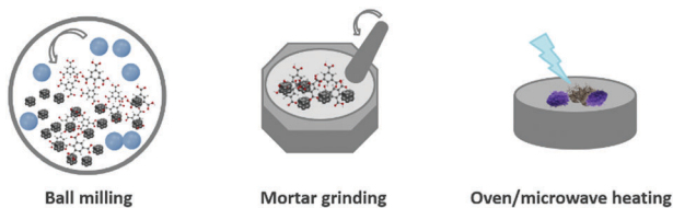
Fig. 3 Schematic diagrams illustrating the solvent-free synthesis of MOFs from solid matters.
