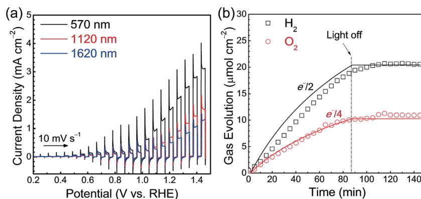
Fig. 4 (a) Current–potential curves obtained from  $\text{Ta}_3\text{N}_5$  photoanodes with different film thicknesses under simulated AM 1.5G light, and (b) time course of  $\text{O}_2$  (open circles) and  $\text{H}_2$  (open squares) gas evolution from a  $\text{Ta}_3\text{N}_5$ (570 nm)/Ta/Ti photoanode held at 1.23 V vs. RHE and a Pt counter electrode, respectively, under simulated AM 1.5G light. Solid curves represent the total charges estimated from the photocurrent.
