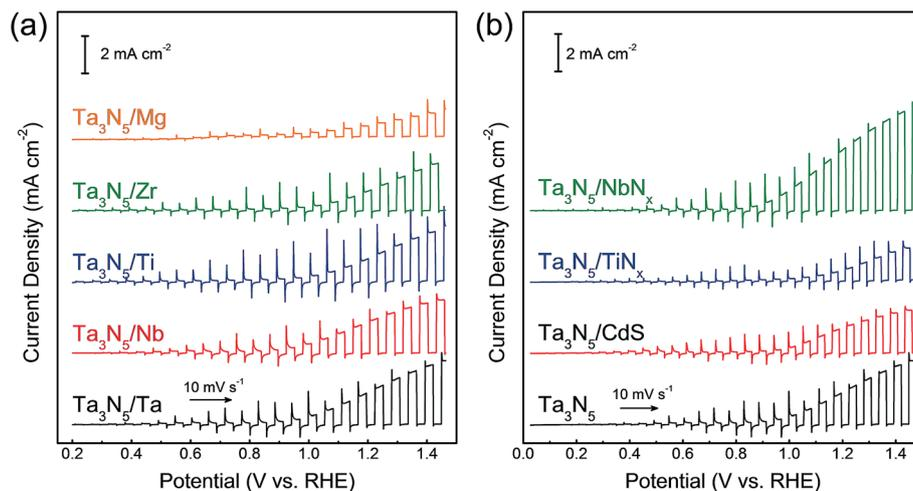
Fig. 5 Current–potential curves obtained from  $\text{Ta}_3\text{N}_5$  photoanodes with different back contact layers. (a)  $\text{Ta}_3\text{N}_5/\text{M}/\text{Ti}$  ( $\text{M} = \text{Ta}, \text{Nb}, \text{Ti}, \text{Zr}$  and  $\text{Mg}$ ), and (b)  $\text{Ta}_3\text{N}_5/\text{N}/\text{Ta}/\text{Ti}$  ( $\text{N} = \text{NbN}_x, \text{TiN}_x$  and  $\text{CdS}$ ).
