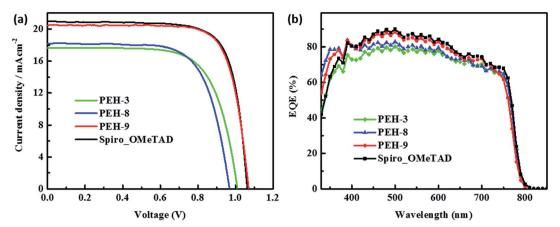
Fig. 5 (a) Current (J) –voltage (V) curves of the solar cells with PEH-3, PEH-8, PEH-9 and Spiro-OMeTAD control recorded from forward bias (FB) to short circuit conditions (SC) under AM 1.5 conditions (100 mW cm<sup>-2</sup>). (b) Incident photon-to-electron conversion efficiency (IPCE) as a function of wavelength for the PSCs in (a).
