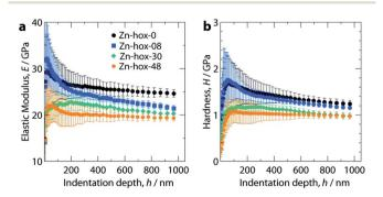
Fig. 4 Elastic moduli, E (a) and hardness, H (b) as a function of indentation depth, h along [110]. With increasing x in  $[NH_3NH_2]_{1-x}$ [NH<sub>3</sub>OH]<sub>x</sub>Zn(HCOO)<sub>3</sub>, the elastic modulus and hardness decrease monotonically due to reduced hydrogen bonding interactions upon substitution.
