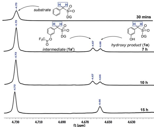
Scheme 2 Reaction profile of *meta*-hydroxylation. <sup>a</sup>Reactions were performed with 1.5 equiv. of  $\text{PhI}(\text{TFA})_2$ .
