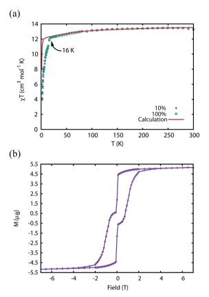
Fig. 2 (a) Magnetic susceptibility temperature product for 2Dy versus temperature measured in a 0.1 T field (field-cooled). Note that the ab initio data was scaled by 0.968 to reproduce the experimental values above 200 K. (b) Magnetisation hysteresis of 2Dy measured at 1.8 K with a sweep rate of 3.5 mT s $^{-1}$ . Saturation of the magnetisation at a value of 5.1  $\mu_{\rm B}$  is indicative of a  $|\pm15/2\rangle$  ground state.
