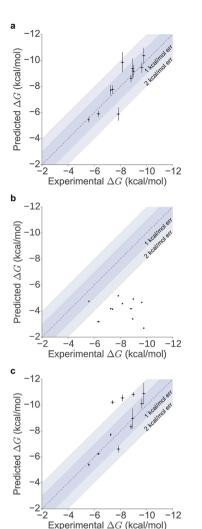
Fig. 5 Scatter and correlation plots of the results. Correlation plots for (a) the free energy calculations starting from the X-ray structures, (b) the docking free energy scores and (c) the free energy calculations starting from the docked structures.
