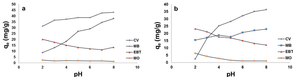
Fig. 8 Effect of pH on the adsorption capacity ( $q_e$ ) of model dyes onto: [a] MSP NPs and [b] MP NPs. Adsorbent:  $2 \text{ g L}^{-1}$ , dyes  $100 \text{ mg L}^{-1}$ , temperature:  $25 \text{ }^\circ\text{C}$ , time: 120 min. Magnetite/Pectin Nanoparticles: MP NPs and Magnetite/Silica/Pectin Nanoparticles: MSP NPs.
