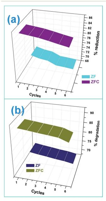
Fig. 10 (a) Reusability of ZF and ZFC for Cr(v) reduction and (b) reusability of ZF and ZFC for 4-CP degradation under solar light.
