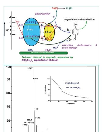
Fig. 9 (a) Band gap structure for the  $ZrO_2-Fe_3O_4$  heterostructure and mechanism of Cr(v) reduction and 4-CP removal and (b) mass spectrum of the solution containing 4-CP after 1 hour of degradation under solar light in the presence of ZFC (inset: COD removal in the presence of ZFC).
