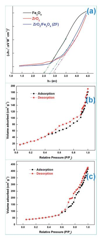
Fig. 5 (a) Tauc plots, (b)  $N_2$  adsorption–desorption isotherms for ZF and (c)  $N_2$  adsorption–desorption isotherms for ZFC.
