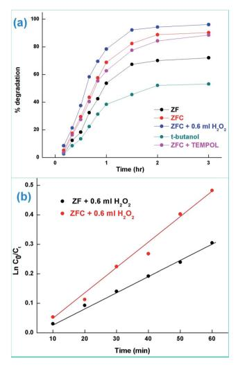
Fig. 8 (a) Degradation of 4-CP under solar light and (b) kinetics plots for 4-CP degradation by ZF and ZFC in the presence of  $\rm H_2O_2$  under solar light (initial pH = 5.5, initial conc. of 4-CP = 20 mg L<sup>-1</sup>, and temperature = 30  $\pm$  0.5 °C).
