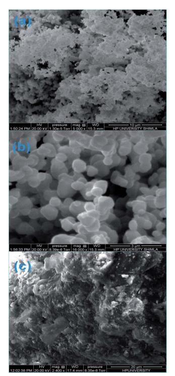
Fig. 3 (a) Low resolution SEM image of ZF, (b) high resolution image of ZF, and (c) SEM image of ZFC.
