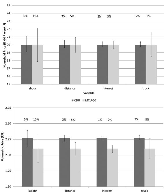
Fig. 8 Sensitivity analysis of labour, distance, interest, and 5 tonne truck when collection rates are set to 1.8 L HH<sup>-1</sup> day<sup>-1</sup> for household cost (top) and volumetric cost (bottom). Solid bars indicate original value, error bars indicate range of values due to sensitivity modelling. Percentage changes are indicated above original values.
