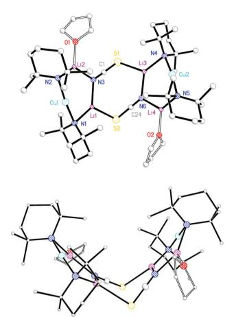
Fig. 4 (a) Molecular structure of 10<sub>2</sub>. H-atoms omitted. Selected bond lengths (Å) and angles (°): N1-Cu1 1.908(2), N2-Cu1 1.906(2), N1-Li1 1.977(5), N2-Li2 1.995(6), S2-Li1 2.500(6), N3-Li1 2.071(6), N3-Li2 2.105(6), N3-C1 1.159(4), S1-C1 1.627(3), Cu1-N1-Li1 87.45(18), Cu1-N2-Li2 87.66(18), N1-Li1-N3 130.7(3), N2-Li2-N3 128.9(3), Li1-N3-C1 125.0(3), Li2-N3-C1 124.8(3), S2-Li1-N3 108.8(2), Li1-S2-C24 91.72(17); (b) view emphasising the boat-shaped dimer core.
