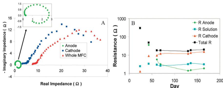
Fig. 8 (A) Nyquist plots showing a significant contribution of cathode impedance to the total impedance of MFC; and (B) behaviors of anode, cathode and solution membrane impedance over time during the enrichment of exoelectrogens in the MFC (Reprinted with permission from ref. 126. Copyright 2010 American Chemical Society).
