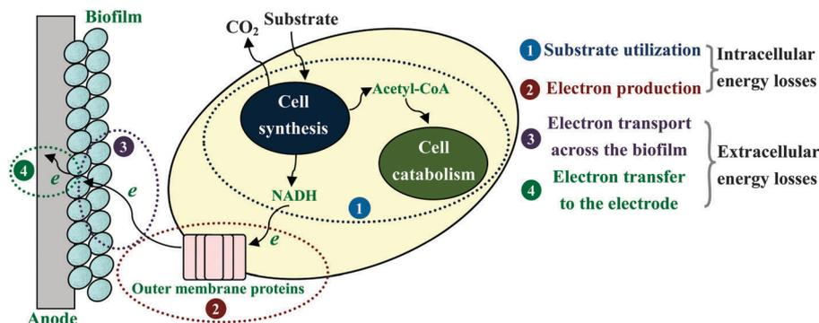
Fig. 6 Schematic of the electron transfer process at the anode of MFC with sequential energy losses.
