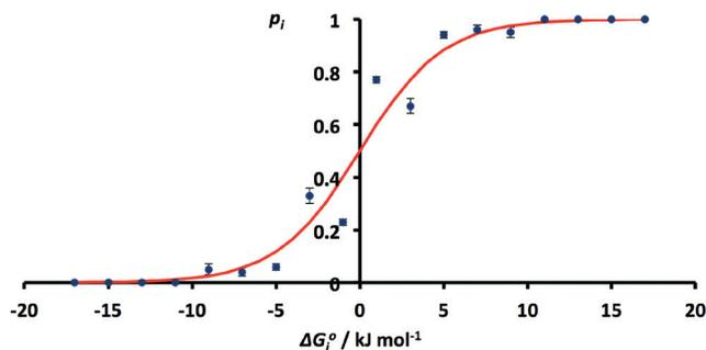
Fig. 6 Relationship between  $\Delta G_i^0$  and  $p_i$  obtained by summing H-bond populations over  $2 \text{ kJ mol}^{-1}$  windows in  $\Delta G_i^0$  (RMSE = 0.07). The red line corresponds to the Boltzmann distribution in eqn (5).
