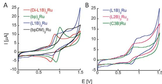
Fig. 3 Comparison between the cyclic voltammograms of (A) 0.5 mM intermolecular Ru complexes and (B) 0.5 mM (**L1B**)<sub>3</sub>Ru and (**C3B**)Ru and 0.25 mM (**L2B**)<sub>3</sub>Ru<sub>2</sub> that were recorded in acetonitrile at rt. using a glassy carbon working electrode, platinum counter electrode, and Ag/AgNO<sub>3</sub> reference electrode. Scan rate: 100 mV s<sup>-1</sup>.
