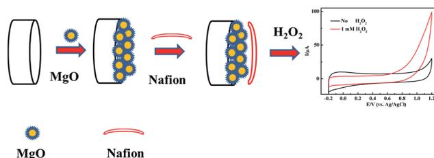
Fig. 1 Schematic diagram of the electrochemical H<sub>2</sub>O<sub>2</sub> sensor.
