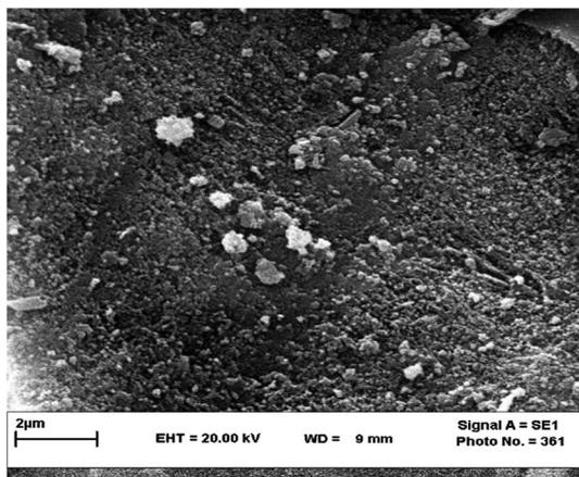
Fig. 5 SEM image of finely powdered cuttlebone.
