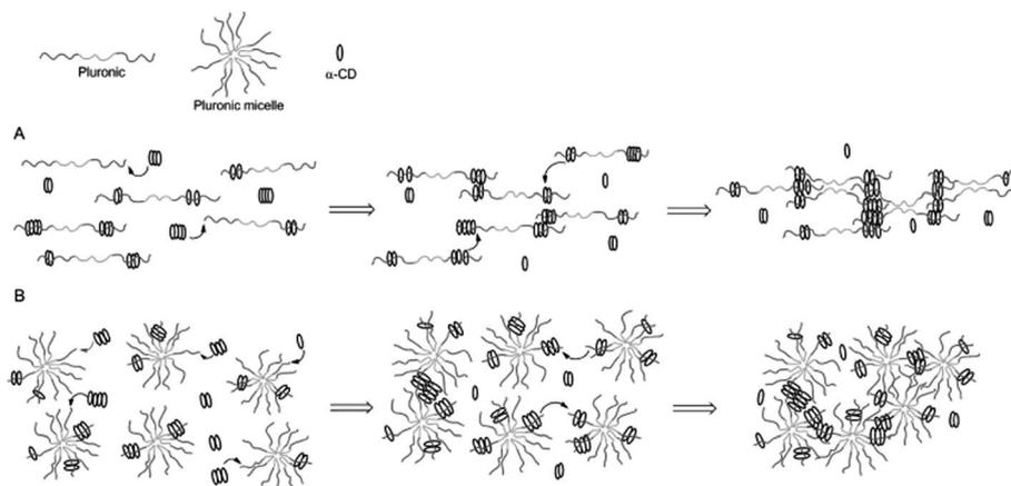
**Fig. 10** Temporal gelation mechanism of linear Pluronic (*e.g.*: F6810 and F6820) or Pluronic micelles (*e.g.*: F12710) and  $\alpha$ -CD. (A) Gelation without micelle formation. (B) Gelation in the presence of micelles. Reprinted with permission from.<sup>104</sup> Copyright 2013, American Chemical Society.
