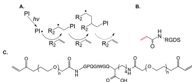
Fig. 1 (A) Schematic of chain-growth photopolymerization for forming peptide-immobilized hydrogels (PI: photopolymerization,  $h\nu$ : light source). (B) Acrylated RGDS peptide for co-polymerization into PEGDA hydrogels. (C) Schematic of an acrylate-PEG-GPQGIWGQ-PEG-acrylate crosslinker.
