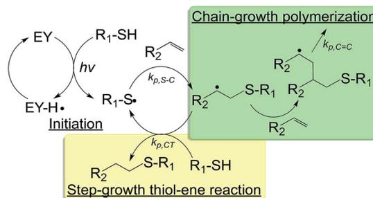
Fig. 3 Schematic of a visible light initiated mixed-mode photopolymerization for forming hydrogels (EY: eosin-Y;  $h\nu$ : visible light source;  $k_{p,S-C}$ ,  $k_{p,C=C}$ ,  $k_{p,CT}$ : kinetic constants for thiol-carbon radical propagation, carbon-carbon radical propagation, and chain-transfer, respectively).<sup>56</sup>
