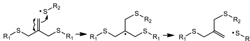
Fig. 6 Mechanism of addition fragmentation chain transfer of an allyl sulfide functional group upon attack by a thiyl radical. Redrawn with permission from.<sup>84</sup> Copyright 2014, John Wiley and Sons.
