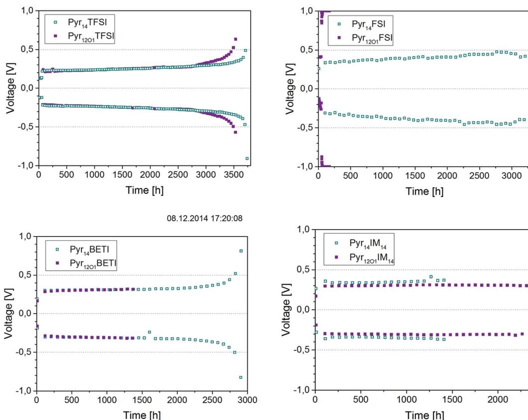
Fig. 9 Stripping–plating in symmetrical lithium cells at  $0.1\text{ mA cm}^{-2}$  and  $40\text{ }^{\circ}\text{C}$ . The ionic liquid present in the electrolytes is indicated in the legends.
