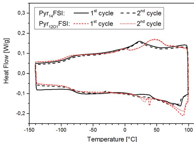
Fig. 6 DSC curves of Pyr<sub>14</sub>FSI- and Pyr<sub>1201</sub>FSI-containing electrolytes, 1<sup>st</sup> and 2<sup>nd</sup> heating/cooling cycle, exothermic heat up.
