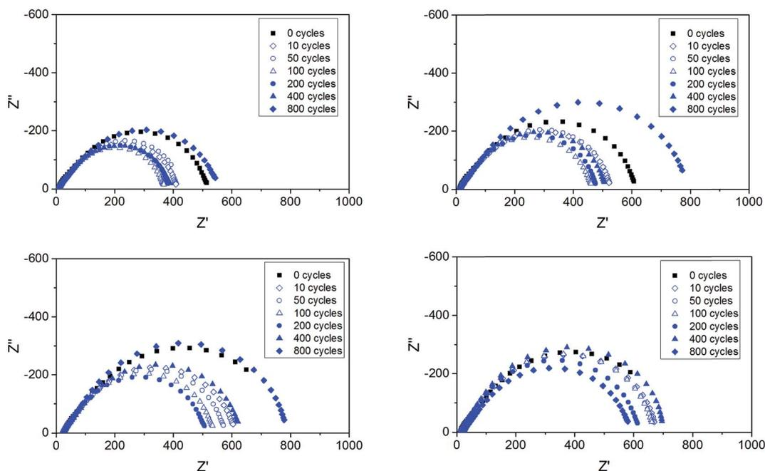
Fig. 10 Electrochemical impedance spectra of ternary electrolytes containing  $\text{Pyr}_{14}\text{TFSI}$  (left, top) and  $\text{Pyr}_{1201}\text{TFSI}$  (right, top),  $\text{Pyr}_{14}\text{BETI}$  (left, bottom) and  $\text{Pyr}_{1201}\text{BETI}$  (right, bottom) recorded at 21  $^{\circ}\text{C}$  during the plating–stripping cycle test at 40  $^{\circ}\text{C}$ . Frequency range: 100 kHz–1 Hz.
