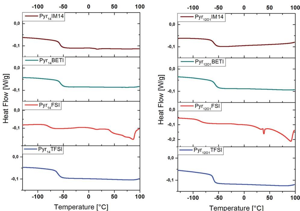
Fig. 4 DSC of polymer electrolytes, 5 K  $\text{min}^{-1}$ , 1<sup>st</sup> heating scan, exothermic heat up.
