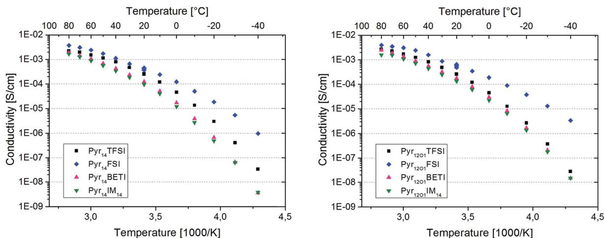
**Fig. 5** Arrhenius plot for Pyr<sub>14</sub> – (left side) and Pyr<sub>12O1</sub> – (right side) containing electrolytes.
