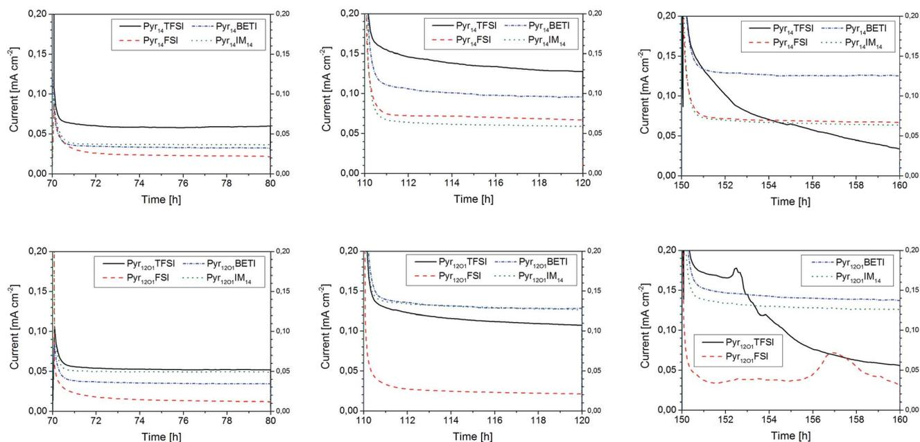
Fig. 7 Chronoamperometry curves upon 10 h polarization steps (intermixed with 10 h relaxation steps) at 0.2 V (left), 0.6 V (center) and 1.0 V (right); Pyr<sub>14</sub>-containing electrolytes (top) and Pyr<sub>1201</sub>-containing electrolytes (bottom). All measurements were performed at 40 °C.
