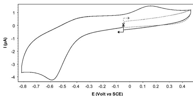
Fig. 4 Cyclic voltammogram of Cu(II)@3 recorded under argon in water (NaNO<sub>3</sub> (0.1 M), NaOH (1.5 mM)) (carb.,  $\varnothing$  = 3 mm;  $\nu$  = 0.05 V s<sup>–1</sup>).
