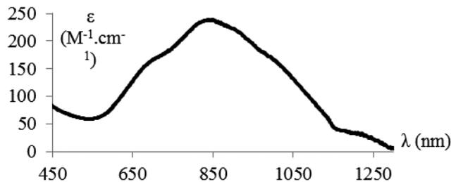
Fig. 2 Near-IR/vis spectrum of Cu(II)@3 (H<sub>2</sub>O–NaOH, pH ≈ 8, 298 K).
