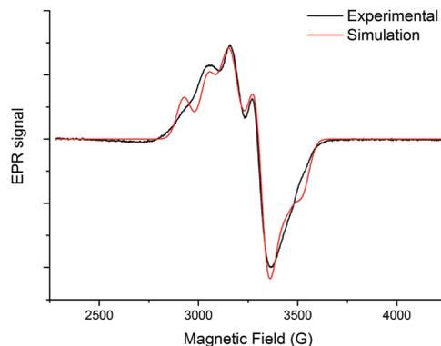
Fig. 3 EPR spectra of Cu(II)@3 in frozen water solution (H<sub>2</sub>O–NaOH, pH ≈ 8, *T* = 70 K) (black line: experimental spectra; red line: simulated spectra). Experimental conditions:  $\nu$  = 9.655 GHz, power = 2 mW and modulation amplitude = 2.0 G. Best fit parameters:  $g_1$  = 2.015,  $g_2$  = 2.135 and  $g_3$  = 2.220,  $A_1$  = 193 MHz,  $A_2$  = 158 MHz and  $A_3$  = 363 MHz for a lwpp = 70 G Gaussian lineshape.
