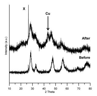
Fig. 1 pXRD pattern of Cu/HSACeO<sub>2</sub> catalyst before and after reaction. Only one peak can be tentatively assigned to a Cu or CuO phase either before or after reduction. The pattern for the catalyst after reaction indicates a more amorphous structure possibly due to the formation of  $Ce_2O_3$  phases [The sharp peak at 26  $2\theta$ ° X is from the brass insert used in the sample holder].
