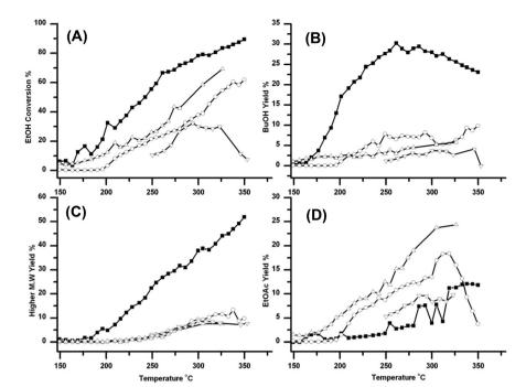
Fig. 5 Summary of the effect of pressure and the presence of  $CO_2$  on the reaction over  $Cu/HSACeO_2$ . The traces show as follows (A) conversion of EtOH (B) yield of BuOH (C) yield of  $>C_4$  products and (D) yield of EtOAc. In each plot the points are labelled as follows: (without  $CO_2$ ) = 100 bar, = 30 bar, = atmospheric pressure, and the result of 100 bar = 100 b
