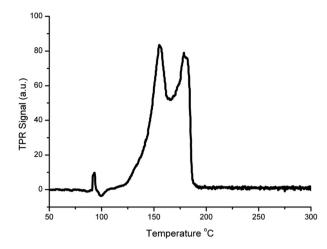
Fig. 2 Results of temperature programmed reduction of the unreduced Cu/HSACeO2 catalyst immediately following calcination; two well separated peaks can be seen at 155 and 178 °C, these two peaks are tentatively assigned to non-crystalline CuO interacting with CeO<sub>2</sub> and larger non-crystalline CuO associated with CeO2 respectively.
