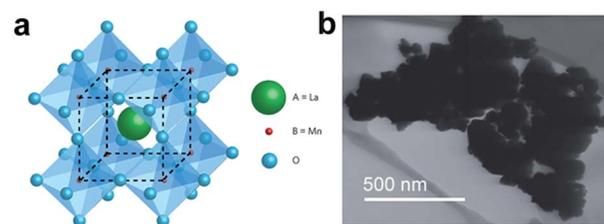
Fig. 3 (a) Idealized cubic  $\text{LaMnO}_3$  perovskite structure. (b) Dark-field SEM image of  $\text{LaMnO}_{3.09}$  nanoparticles. Reproduced with permission from ref. 25. Copyright 2014 Macmillan Publishers Limited.
