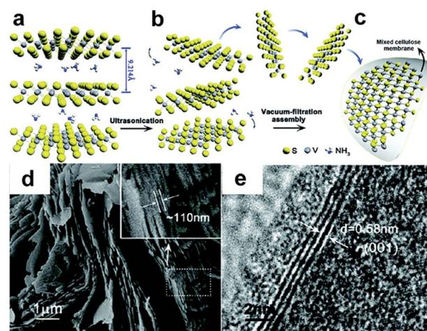
Fig. 13  $\text{VS}_2$  nanosheets for supercapacitor electrodes. S–V–S multilayers with intercalated  $\text{NH}_3$  molecules (a) is used to exfoliate thin layers of  $\text{VS}_2$  (b). The transfer is accomplished by vacuum filtration and the layers are transferred on mixed cellulose membranes (c). SEM (d) and HR-TEM (e) images of the multilayer with  $\text{NH}_3$ . Reproduced with permission from ref. 158. Copyright 2011 American Chemical Society.
