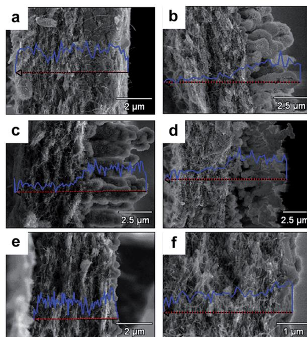
Fig. 21 Cross-section morphologies and X-ray line scan spectra of Mn element in pristine composites (MCM0), and after 500 cycles at  $20 \text{ mV s}^{-1}$  (MCM20),  $60 \text{ mV s}^{-1}$  (MCM60),  $100 \text{ mV s}^{-1}$  (MCM100),  $300 \text{ mV s}^{-1}$  (MCM300), and  $500 \text{ mV s}^{-1}$  (MCM500). (a) MCM0, (b) MCM20, (c) MCM60, (d) MCM100, (e) MCM300, and (f) MCM500. Reproduced with permission from ref. 232. Copyright 2012 Elsevier.
