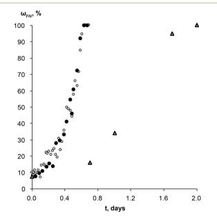
Fig. 7 Weight fraction of the theophylline form IV in the SMPT from theophylline form II/form IV mixture ( $w_{II}/w_{IV}$ ; 90/10) to form IV, in saturated (○) form IV and (●) form II methanol solutions at 23 °C. △ represents the weight fraction of the theophylline form IV in the solid phase during the SMPT from theophylline form II in methanol at 23 °C. All kinetic curves are aligned to the point when solid phase of respective SMPT contained 10% of form IV.
