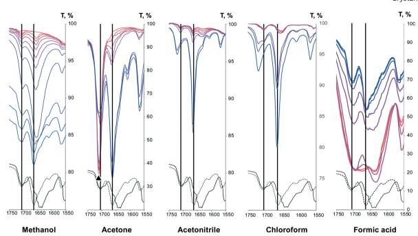
Fig. 12 FTIR spectra of carbonyl group stretching band region during theophylline crystallization from saturated solutions upon solvent evaporation at room temperature. Colour gradient shows FTIR spectra changes throughout crystallization (red – saturated solution, blue – crystallization product). FTIR spectra of solid theophylline form II (dashed line) and IV (continuous line) are added for comparison purpose. Acetone carbonyl group stretching band is marked with ▲.
