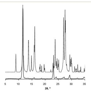
Fig. 4 PXRD patterns of form IV obtained by SMPT in methanol (solid line); and simulated from crystal structure (dashed line).
