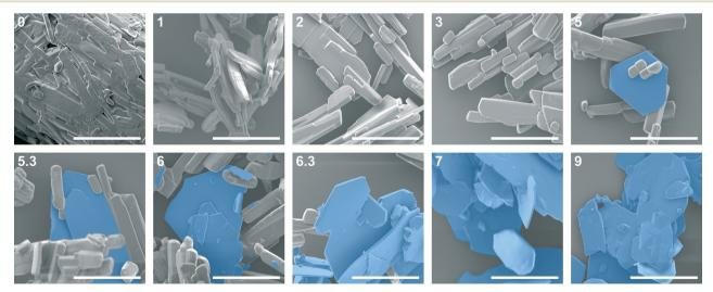
Fig. 3 SEM images throughout SMPT from theophylline form IV in methanol at 23  $^{\circ}$ C. Inset: time of sample gathering (days); 40  $\mu$ m scale bar, crystals of theophylline form IV indicated with blue colour.
