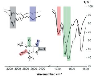
Fig. 11 FTIR spectra of theophylline form II (solid line) and form IV (dashed line), showing carbonyl group, alkene group hydrogen bond and imidazolium group hydrogen bond stretching band assignment.
