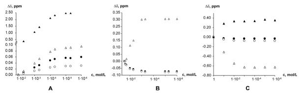
Fig. 9 Theophylline chemical shift displacement depending on chloroform-D (A); deuterium oxide (B); and formic acid-D2 (C) concentration. Chemical shifts are indicated as: methyl group C10 protons (•); methyl group C12 protons (ο); alkene group proton (C8–H) (Δ); and imidazolium group proton (N7–H) (Δ).
